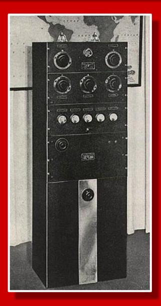
This was a floor-standing 100 watt phone and CW transmitter that was designed to replace the aging 150 series. **The November 1934 QST ad stated:** *<u>"It's ultramodern dress will lend an</u> <u>air of distinction to anyone's library."</u> Introduced in one of the last B/W ads.*
