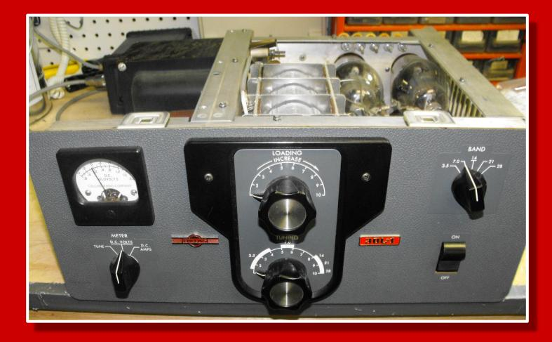
**COLLINS PROMOTIONAL** TEXT - "The Collins 30L-1 has 1000 watts PEP power input on SSB and 1000 watts average on CW on 80, 40, 20, 15 and 10 meters. Uses TWO FINALS (811A) Drive power is 70 to 100 watts for full power output. RF connection is N type." (Ask Don Crosby about his)
