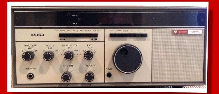
"The 451-S is a professional single sideband (SSB) communications receiver that offers reception of upper and lower sideband, CW, AM, or FSK signals over the frequency range of 0.2 to 30 MHz. The unit is of solid-state design ... and uses single know tuning to cover the entire frequency range without band switching. A high resolution synthesizer with microprocessor controls four tuning rates down to 10 Hz increments."
