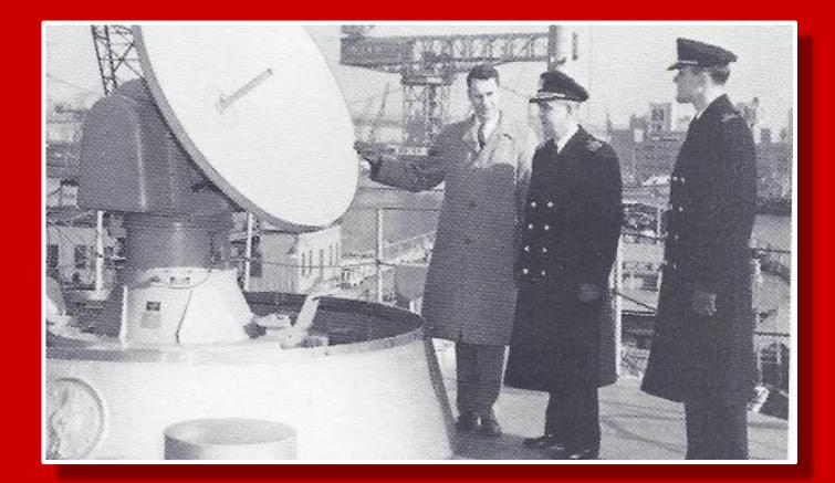
"The ship's navigator can find his position just as if he had an assistant watching the sun through an ordinary extant. No cloudy weather gets in the way of the radio sextant, nor can an enemy jam the radio impulses (as is possible with other radio aids to navigation, such as Loran."
