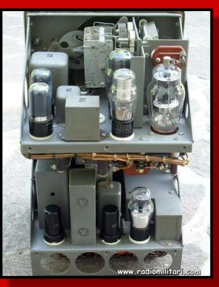
Frequency Coverage: 2 to 16 MHz in three bands A-2 to 4 MHz 10 watts trans. B-4 to 8 MHz C-8 to 16 MHz F: 455 KHz Tubes rx : 2 x 12SK7, 1 x 12SA7, 1 x 12SQ7, 1 x 6G6G Tubes tx : 3 x 6V6G, 1 x 807, 1 x VR-150-30 Dimensions: 14 ¼ H x 9 5/8 W x 9 ¾ D inc. Transmitter Weight: 10 lb. Power supply: Dynamotor 415E 12V Manual: Collins
