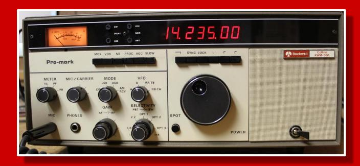
large and heavier than other transceivers. It contains a speaker, power supply, second VFO, and space for a host of accessory items such a unique type of new speech processor."
