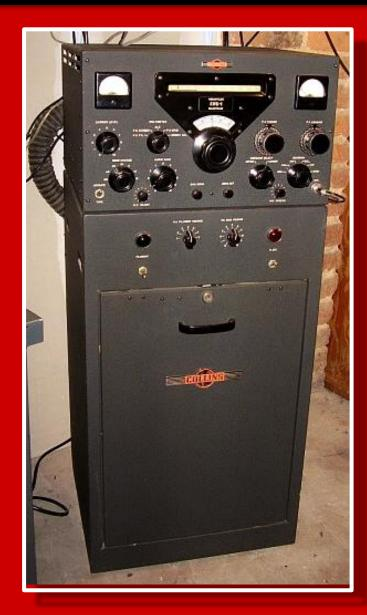
**COLLINS PROMOTIONAL TEXT –** "The most advanced design features ever offered in an amateur transmitter ... unprecedented compactness is achieved without crowding, *the exciter* and RF power amplifier are housed in a single receiver-size cabinet which can be place on the operating desk or mounted on of the power supply cabinet.
