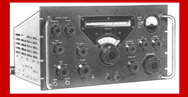
"The Collins 51J-4 Receiver is designed for communication applications where stability and dial accuracy of the highest order are the prime requisites. Under normal operating conditions, the receiver operates in the range of 540 kc to 30.5 mc with a total setting error and *drift of less than 1 kc at any frequency* within its range. This receiver incorporates the new mechanical filter in the intermediate frequency range to obtain the desirable rectangular-shaped passband.
