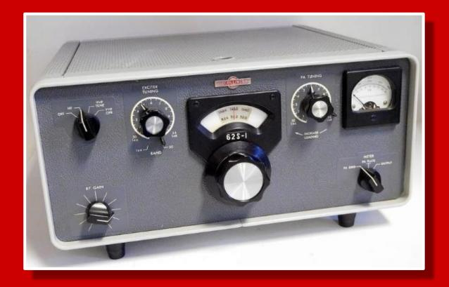
COLLINS TEXT – "The Collins 62S-1 permits you to enjoy operation on either 6 or 2 meters by simply snapping a switch. No cable patching is required. It can be used in any operational mode, as determined by the companion receiver and transmitter. Power input is 160 watts.
