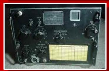
The TCS was designed by Collins and used, along with its matching transmitter and a power supply, during World War II on <u>LST landing</u> <u>craft, P-T boats, and a variety of</u> <u>other smaller boats as well as on-</u> <u>shore applications</u>.
